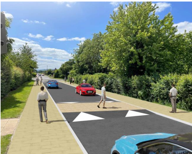
Image: Artist's impression of proposed new raised crossing outside Haddenham Medical Centre
